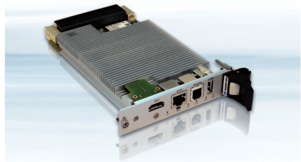
Figure 7: VX3058 single board computer with 8 and 10 Gbits/s port
