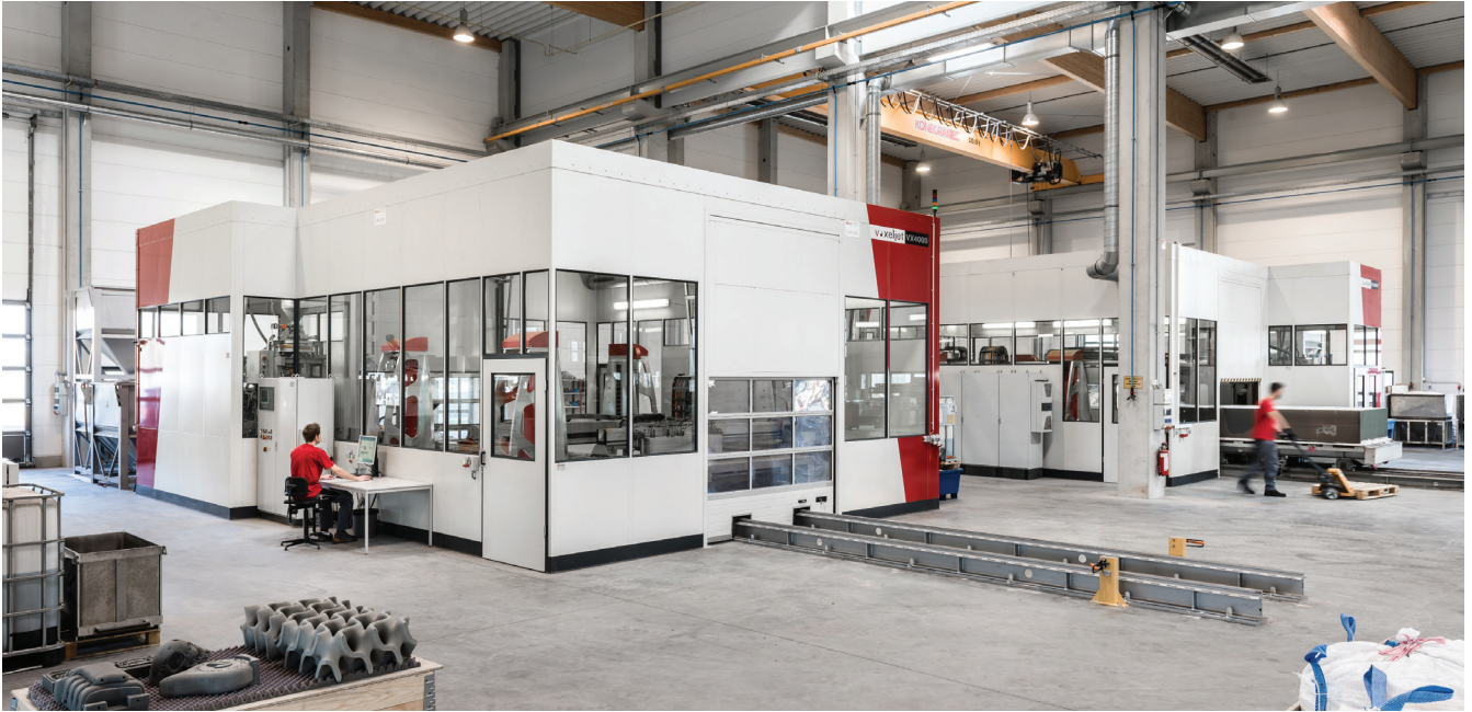
// THE BIGGEST INDUSTRIAL 3D PRINTING SYSTEM FOR SAND MOLDS IS LOCATED IN THE SERVICES HALL OF voxeljet IN FRIEDBERG (BAVARIA). IT COMES WITH A CONTIGUOUS CONSTRUCTED SPACE (LxWxH) OF 4.000 x 2.000 x 1.000 mm. ITS HIGH QUALITY COMPONENTS ARE MADE FOR CONTINUOUS OPERATION. (SOURCE: voxeljet AG)
