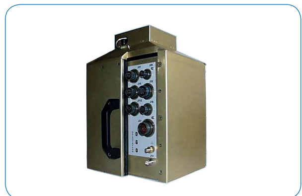
Image 3: The control computer is based on the Kontron PC/104-Plus SBC MICROSPACE® MSM800SEL and the framegrabber MICROSPACE® MSMG104.
