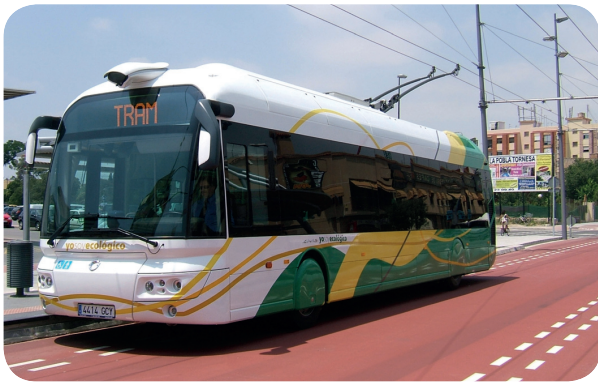
Image 1: By using road markings the Siemens Optiguide steers the bus automatically to within 5 cm of the bus stop.
